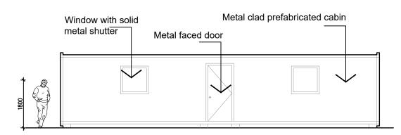
Front Elevation of welfare and storage cabin (no doors or windows on rear elevation).
