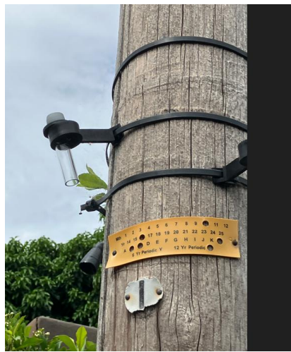
Figure 10 - NO 2 diffusion tube attached to a telegraph post in Bromley
