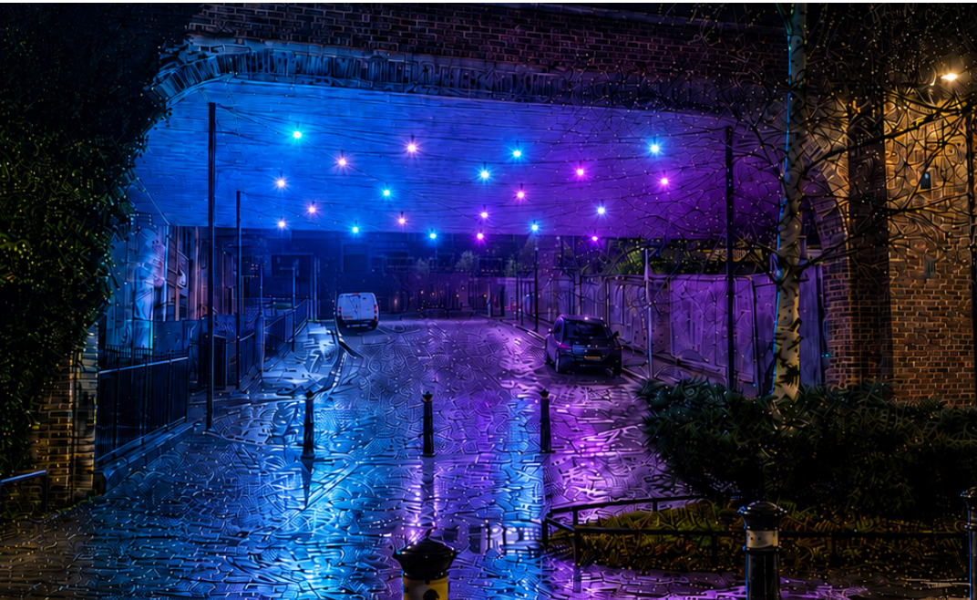
Study 2: Pole mounted catenary
